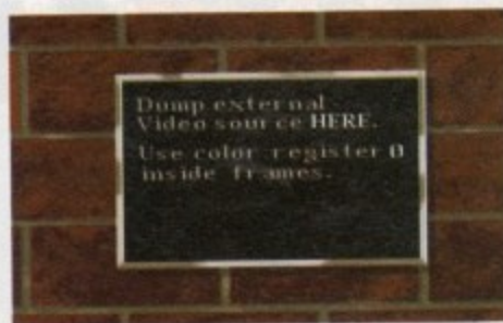
It looks pretty dull here, but that black area will be replaced with the incoming video signal when you connect up a genlock.
